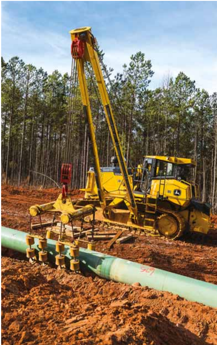
The John Deere-designed and manufactured 1050K PL crawler is available in two configurations for 170 000 lb (PL170) and 220 000 lb (PL220) of maximum lift capacity.
