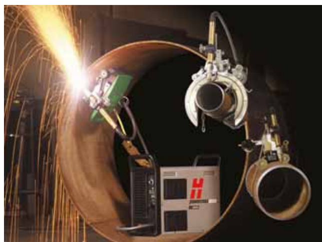
Figure 4. Automated pipe cutting machines like this one from Mathey Dearman are making it easy for pipeline contractors to make smooth and accurate bevelled edges using plasma.
