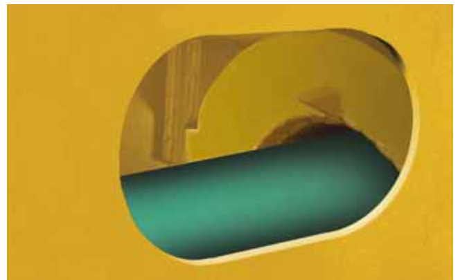
Innovative 'peek-a-boo' window in the Standard 6 - 20 in. bender.
