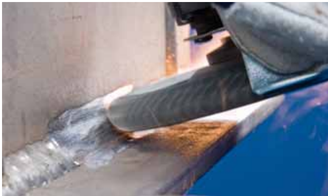
Figure 2. POLIFAN®-CURVE radial flap disc easily reaches into fillet welds for a smooth finish.
