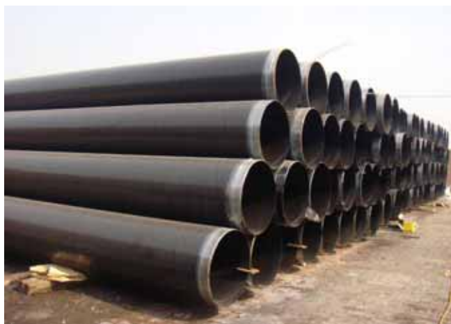
Figure 1. Yard storage of recently coated pipe.
