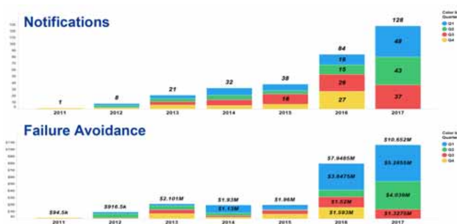
Figure 2. Failure avoidance costs for TransCanada’s Enterprise Analytics anomaly detection. Estimates were calculated conservatively on the basis of a commercial impact of 30% the current parts and labour.
