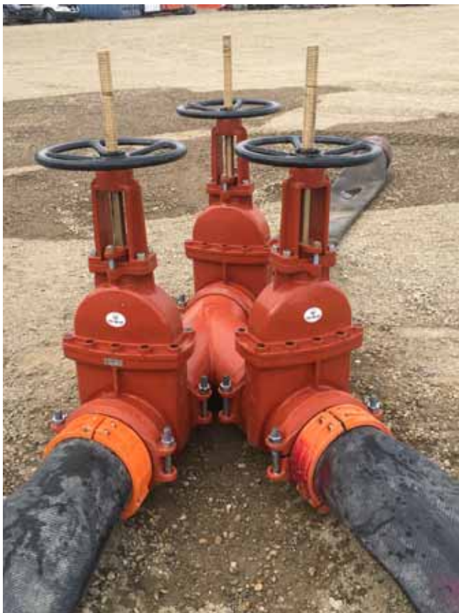
Figure 1. Victaulic pig launcher: a lighter union at every joint for easy disassembly and transportation.
