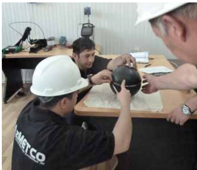
Figure 1. Inspection and measurement of the sphere of the piston prover is part of the calibration procedure.
