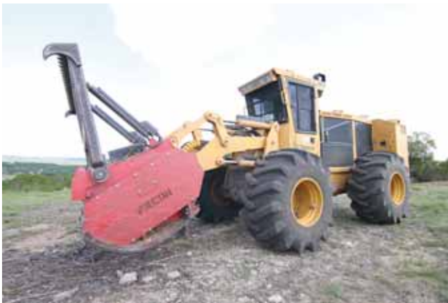
The 300 hp Cedar Eater mulchers are equipped with an 8 ft wide Fecon cutting head that rotates at 1800 rpm.
