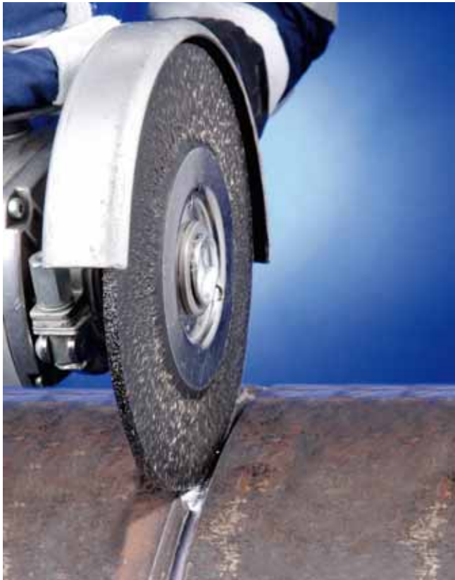
Figure 3. PFERD’s ECAP® brush gets into tight bevels, even on heavy wall pipe.
